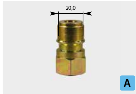
Plug : F. Zinc-plated steel. Max. 250 bar / 150 °C
