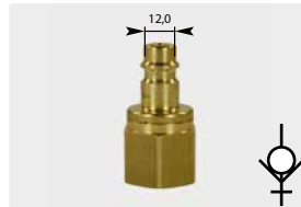
Plug : F. ∅ 12 mm. Brass. With valve. Max. 35 bar / 100 °C
