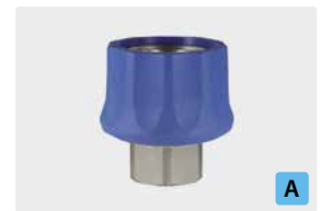
Coupling : F. Nickel-plated brass. Max. 250 bar / 150 °C
