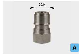
Plug : F. Stainless steel. Max. 250 bar / 150 °C
