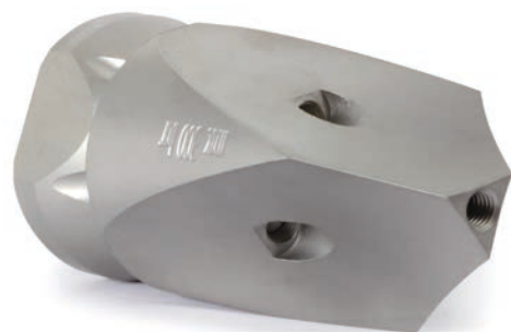
350 bar. 1/4" F. For tubes > 30 mm. Lateral front jets 0.5 mm drilled
