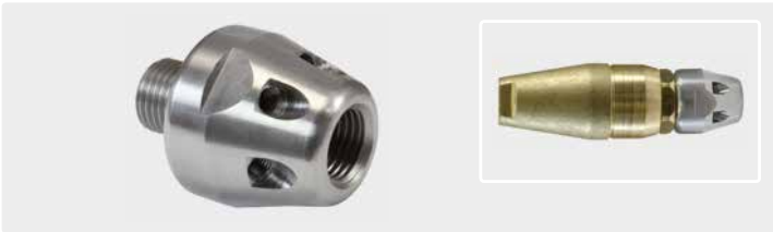
For ST-357/ST-456 rotating nozzles. Hardened stainless steel. Max. 350 bar. \varnothing 1/4" M and 6 M5 threads for nozzle inserts (see table below).
