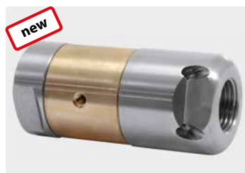
1/2" F. 5 rear jets. 3 side jets. Outside \varnothing 38 mm. Ⓜ 580 g.
