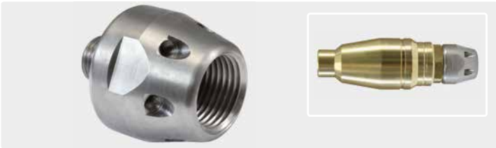
For ST-458/ST-559 rotating nozzles. Hardened stainless steel. Max. 500 bar. \varnothing 1/4" M and 6 M5 threads for nozzle inserts (see table below).
