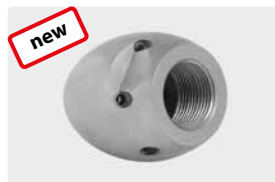
3/4" F. 6x 75° +1x 0°. 30-100 l/min. For \text{R} \text{D} 120-250 mm. Outside \text{D} 50 mm. \text{S} 567 g.
