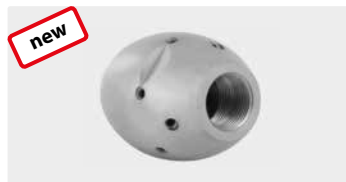
1/2" F. 6x 75° 3x 30° +1x 0°. 80-140 l/min. For \text{R} \text{D} 120-250 mm. Outside \text{D} 40 mm. \text{S} 630 g.
