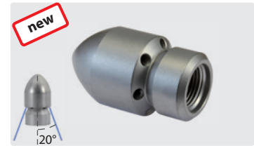
3/8" F. Outside \varnothing 30 mm. 6 rear jets
