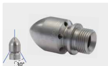
1/2" M. MR cone. Outside \varnothing 30 mm. 6 rear jets, with front jet
