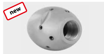
3/4" F. 6x 75° 3x 30° +1x 0°. 100-250 l/min. For \text{R} \text{D} 150-300 mm. Outside \text{D} 50 mm. \text{S} 1,367 g.
