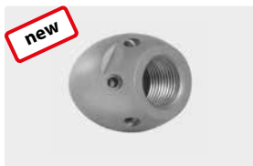
3/8" F. 6x 75° +1x 0°. 25-70 l/min. For \text{R} \text{D} 75-150 mm. Outside \text{D} 35 mm. \text{S} 207 g.
