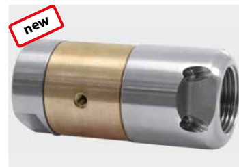
3/4" F. 6 rear jets. 3 side jets. Outside \varnothing 38 mm. Ⓜ 554 g.
