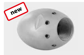
1" F. 8x 75° +1x 0°. 100-250 l/min. For \text{R} \text{D} 150-300 mm. Outside \text{D} 62 mm. \text{S} 1,265 g.
