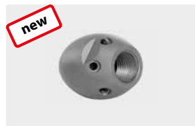
1/4" F. 6x 75° +1x 0°. 20-50 l/min. For \text{R} \text{D} 50-100 mm. Outside \text{D} 30 mm. \text{S} 127 g.
