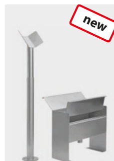
Wash brush holder, two-piece. For floor mounting and positioning for different length of lances. Holder: H x W x D: 315 x 305 x 120 mm. Support pipe: Pipe Ø 42 mm, height adjustable from 570 to 1,000 mm
