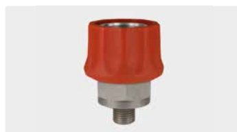
Coupling : M. Stainless steel. Max. 600 bar / 150 °C
