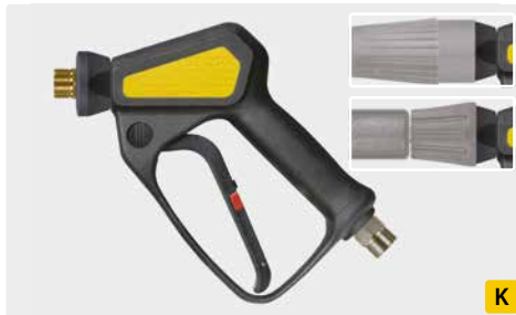
Professional gun with insulated outlet suitable for lances with swivel screw coupling. Max. 310 bar / 45 l/min / 150 °C
