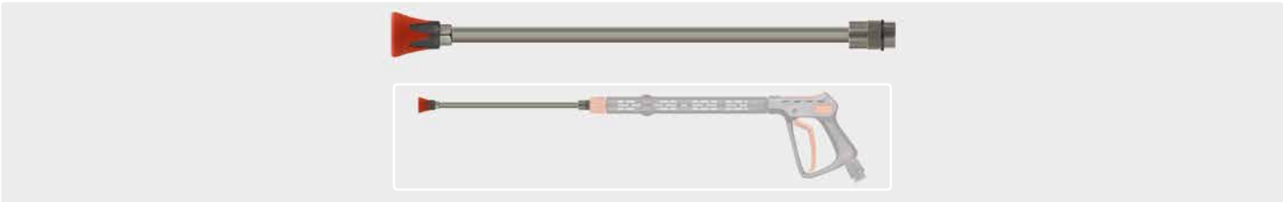
M24 M. Lance 400 mm with nozzle protector ST-10 without nozzle. Lance for ultra high pressure guns with extension ST-9. Max. 600 bar / 150 °C
