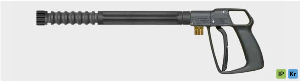
Gun with extension 340 mm and M22 F. Max. 210 bar / 30 l/min / 150 °C
