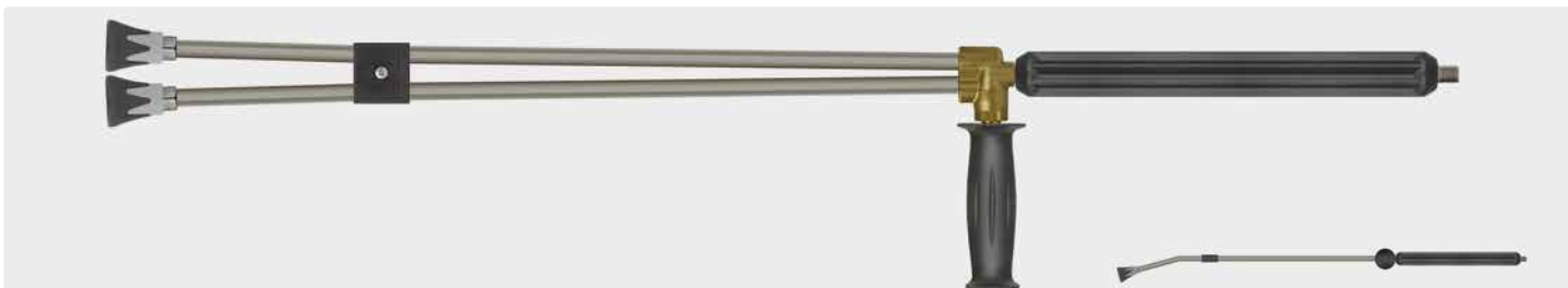
1/4" M. Lance with moulded handle, valve ST-54 and nozzle protector ST-10 with low pressure nozzle &amp; thread 1/4" F. Max. 310 bar / 150 °C
